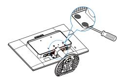
3. Remove the screws from hinge cover.
